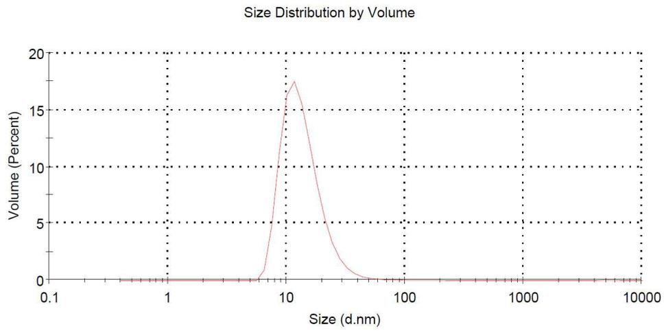
Particle size distribution of the ATO coating solution: DV90 = 21 nm
